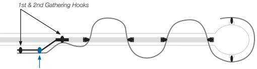
NOTE: An extra gathering hook in one of the spare pockets is used to secure the curtain when an overlap arm is required.
